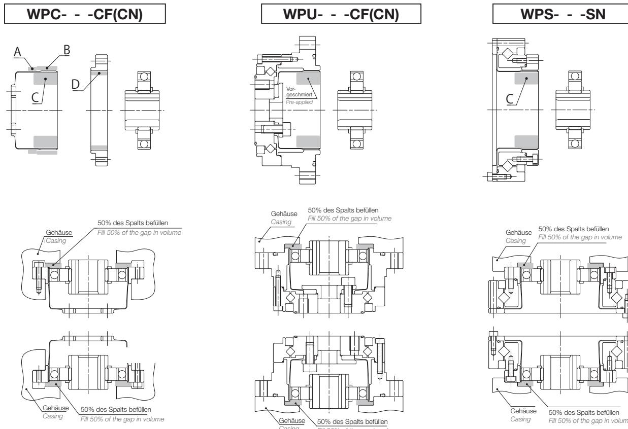
Anforderung an Aufnahmeverrichtung *Attachment fixture requirement***WPC- - -CF(CN)**
